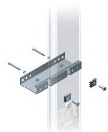
Vertical Shaft Installation
