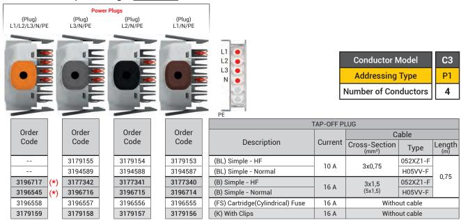
Cable cross-sections in parentheses are used in tap-off plugs marked (\*).
