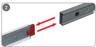
Slide one end of the busbar into the joint module on the other side.
