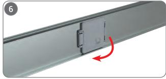
Open the closed plug-in opening cover on the busbar.
