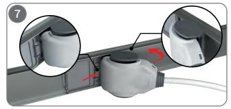
The tap off plug should be installed in the direction as stated in the figure. Tabs which located on the edge of the tap off plug must be installed to the current output windows which located on busbar itself with an angular position. Tap off plug should be positioned parallel to the busbar.
