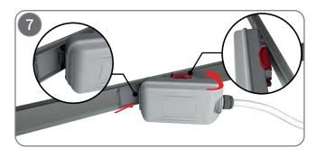
The tap off box should be installed in the direction as stated in the figure. Tabs which located on the edge of the tap off box must be installed to the current output windows which located on busbar itself with an angular position. Tap off box should be positioned parallel to the busbar.
