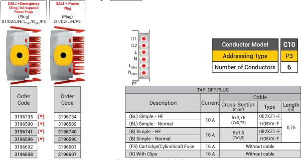
Cable cross-sections in parentheses are used in tap-off plugs marked (\*).
