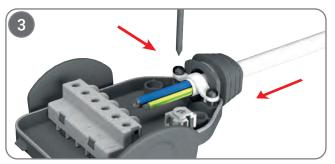
Pass the cable through the cable gland that provides IP protection to the plug and tighten both screws sufficiently by seating the cable clamp into place.
