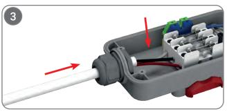
Pass the cable through the cable gland that provides IP protection to the box. Install cartridge (cylindrical) fuses up to a maximum of 32A on 10x38 mm bases.
