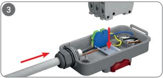
Pass the cable through the cable gland that provides IP protection to the box. Install the miniature circuit breaker (MCB) not exceeding the maximum 32A on the existing DIN rail in the box.
