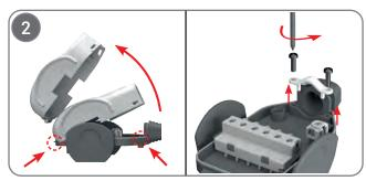
Remove the plug cover as shown in the figure. Remove the cable clamp by unscrewing the two screws.
