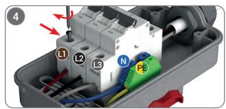
Please connect the yellow protective conductor to the earthing (PE) terminal, the blue neutral conductor cable to the neutral (N) terminal, and the other cables to the relevant phase (L1, L2, L3) terminals. Connect the existing cable ends from the contacts to the input terminals of the MCB in the same way. Complete the operation by tightening the cable gland sufficiently. (Caution: Make sure that the terminal screws are tightened enough.)
