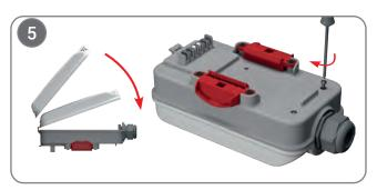
Replace the box cover, turn the box upside down and replace the two screws on the back.
