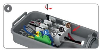
Please connect the yellow protective conductor to the earthing (PE) terminal, the blue neutral conductor cable to the neutral (N) terminal, and the other cables to the relevant phase (L1, L2, L3) terminals. Complete the operation by tightening the cable gland sufficiently. (Caution: Make sure that the terminal screws are tightened enough.)
