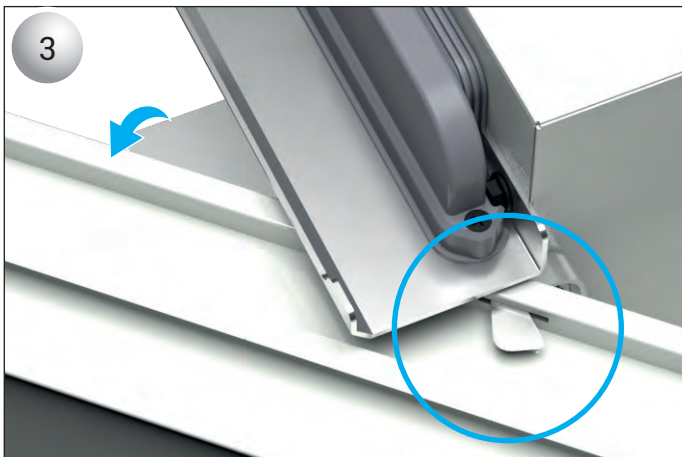
3- After placing the lever plate, move the hanging part of the box towards the body with an angle, and fit it into the place.
