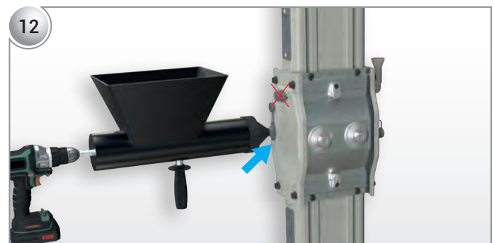
Inject material through the filling hole as shown. Continue filling until Flex-Comp is visible inside the level control plastic.
