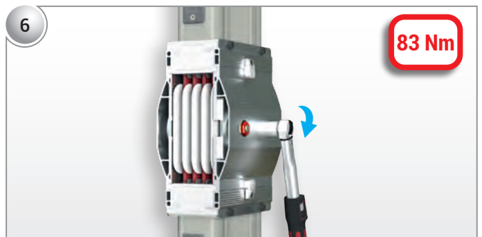
After verifying alignment, torque the block joint nuts to 83 Nm.
