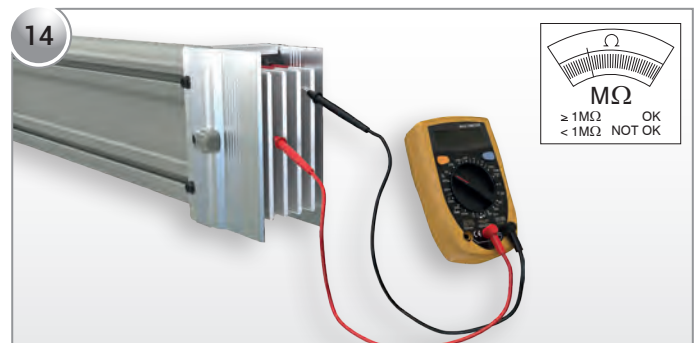
An insulation resistance test must be conducted at least 24 hours after the procedure is completed.
